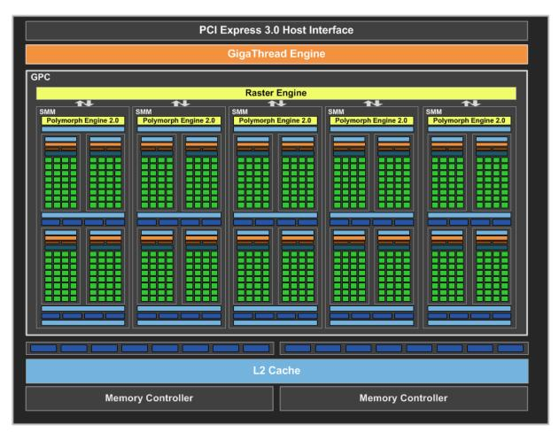
Figure 2: GM107 Full-Chip Block Diagram
