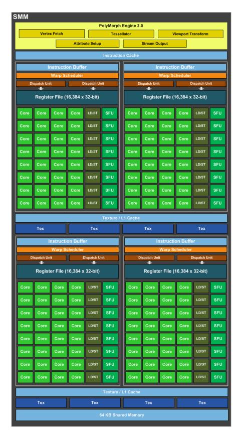
Figure 3: Maxwell SM Block Diagram
