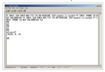
I connected up a level converter board to the UART found earlier. I cut tx coming from the logic board to stop the signals from conflicting. The lag came from minicom, so this interface is instant.
