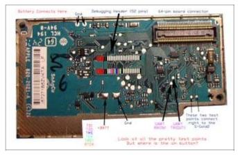
All the JTAG pins are soldered, but the only problem is we don't know how to turn the board on.
