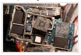
The pads were smaller than I imagined. All the JTAG pads are intact and ready for tracing.
