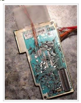
I knew if anyone could do this soldering, it would be my ex-mentor and friend Joe Barbetta. I brought the board down to his shop this morning, and under a microscope with some very fine gauge magnet wire, he soldered it. Thanks.
