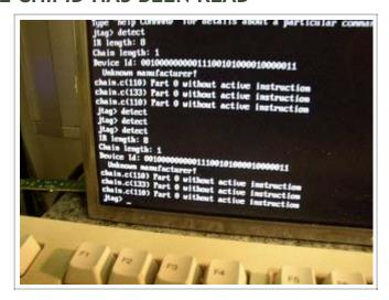
The chipid has been read, so that means the JTAG hardware is working. The first half of the battle is over. I used OpenWinCE to connect, but it doesn't support this chip yet. So now we have to write software for JTAGing ARM926. But we know that the hardware is working!!!
