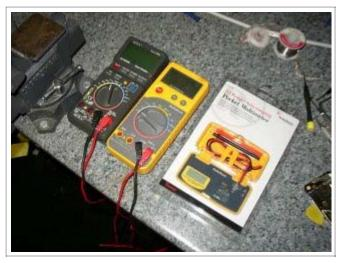
The \$100 multimeters can't beep right away with the continuity check. This \$30 one can.
